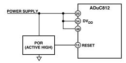
Figure 41. External Active High POR Circuit
